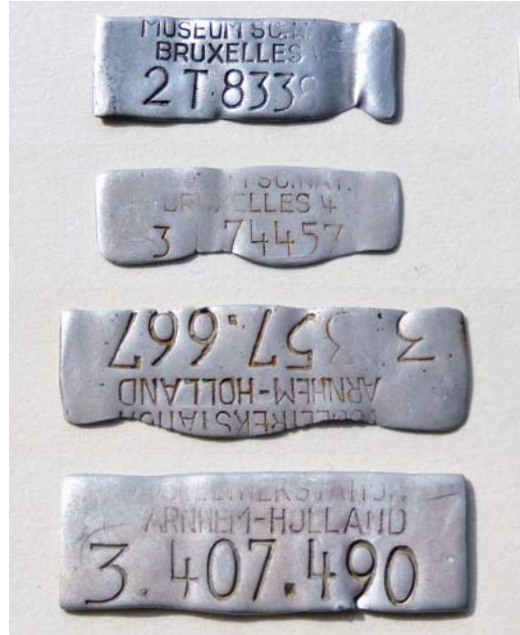
FIGURE 5 Aluminium rings removed from four Black-headed Gulls Chroicocephalus ridibundus breeding on Griend, Friesland, Netherlands (upper three on tarsus, lower on tibia). All trapped on nest and ring replaced by stainless steel ring, Arnhem 3.357.667 upside down; see text for details. Note irregular scalloping of lower edge.
